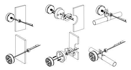
The unit can be surface, flush, or clamp mounted using the included hardware.
