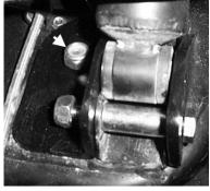
8) Using the 10x110mm bolt attach the bottom of the shock to the lift brackets and stabilizer rod. Place 10mm flat washers on either side of the shock eyelet between the lift brackets.
