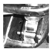
7) Next attach the round backing plate to the underside of the lower control arm buy inserting the 10x40 hex through the backing plate, then through the lower control arm, then through the angle lift bracket. Fasten it tight using the 10mm lock nut.
