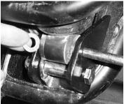
9) Place a small spacer on the outside of the lift bracket then place stabilizer rod eyelet onto the bolt.
