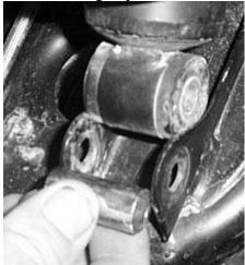
6) Place the appropriate left and right brackets on either side of the shock mount tabs and connect them using a 10x70mm bolt and 10mm lock nut.
