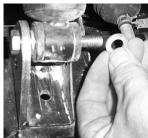
5) Get the 10x110mm bolt and insert it through the large factory washer that was on the outside of the stabilizer link. Next insert the bolt through the stabilizer link eyelet.
