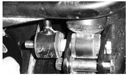
10) Place the large factory washer next to the stabilizer rod eyelet and fasten tight with the 10mm lock nut.
