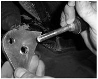
8) Insert the Large Spacer between the shock mount tabs and insert the 10x110mm bolt through the shock mount tabs and spacer. Fasten brackets and both bolts with the 10mm lock nuts.
