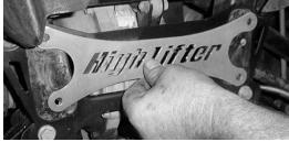
3) Then connect the plate to the frame using 5/16 x 1" stainless steel button head bolts and 5/16 lock nuts.
