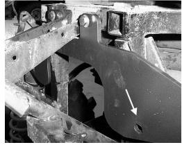
10) You will need to use one large spacer, one small spacer and 10x65mm hex bolt. Place the small spacer between the large lift bracket, the large spacer between the shock mount tabs.
