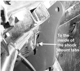
5) Place the Large Spacer into the shock mount tab. Place it between the lift bracket and the shock mount tab.
