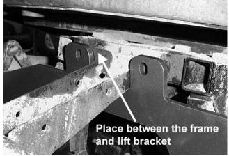
8) Place a small spacer between the lift plate and the plastic support bracket. Secure it a 5/16 x 1 ¼ hex bolts and ¼" flat washers.
