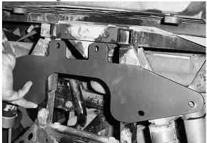
7) Insert the rear plastic support bracket between the long rear lift plate and the frame.
