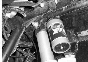
4) Insert one of the front lift brackets into the inside of the shock mount tabs.
