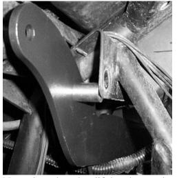
6) Next place the other lift bracket on the outside of the shock mount tabs, to the side that faces the rear.
