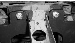
NOTE: Make sure to reconnect the bottom of the plastic support bracket to the frame using the stock hardware.
