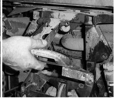
6) Place the large rear lift bracket next to the frame.
