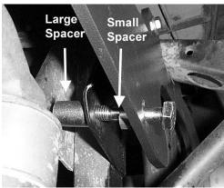
11) Place the small lift plate to the inside of the rear shock mount tabs between the spacer and the shock
