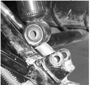
3) Slide bottom of lift bracket over A-arm shock mount and insert one medium spacer between the center of the shock mount tabs and bracket.
