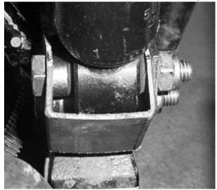
6) Secure the lift bracket to the A-arm using one long brace bracket and one short brace bracket. Sandwich the A-arm with the two brackets with the ½ x 1 ¾ hex bolts and ½" locking nut. Now attach the brace brackets to the top of the lift bracket securing the bracket with the 10mm locking nut.
