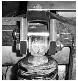
14) Make sure that the brackets run 20 degrees to the shock mount.
