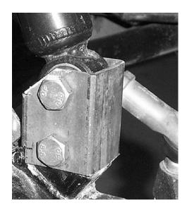
4) Now insert the 10 x 60 hex bolt and secure the bracket and spacer to the frame with the 10mm Locknut.
